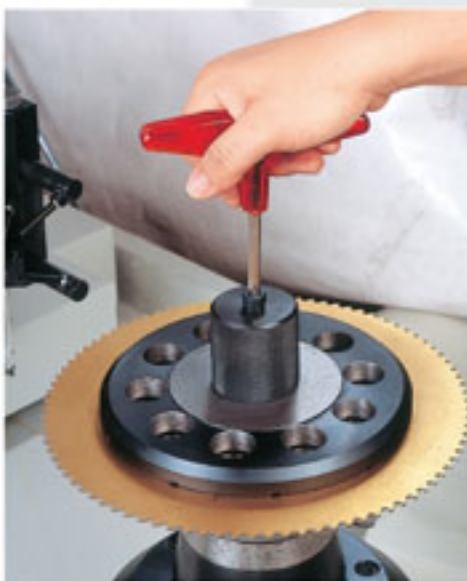
Patented Sawblade Locking Design
